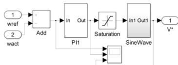
Fig -10: Control circuit of Speed Control of Induction Motor
