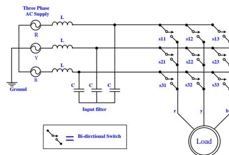
Fig -1: Matrix converter Topology
