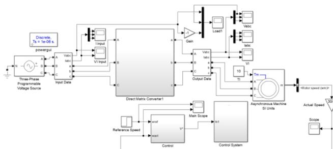
Fig -9: 3-Φ IM Faded 3-Φ to 3-Φ DMC with Closed Loop
