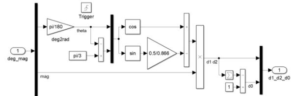
**Fig -19:** Simulink implementation of duty cycle calculation
