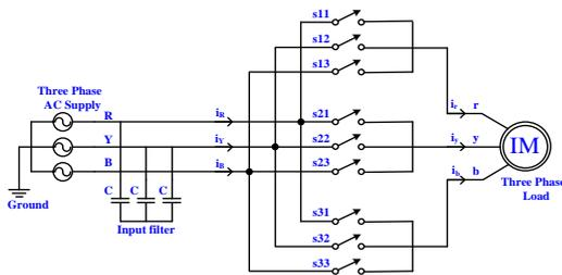
**Fig -2:** Direct matrix converter topology
