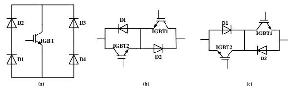
**Fig -4:** (a) Diode Bridge Arrangement (b) Common Emitter Arrangement (c) Common Collector Arrangement
