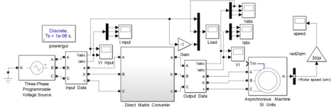
Fig -8: 3-Φ IM faded 3-Φ to 3-Φ DMC with Open Loop
