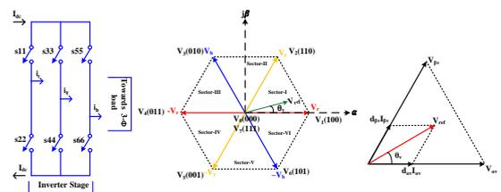
**Fig -7:** (a) VSI stage of of MC (b) Output voltage vector diagram in Hexagon form (c) Sector of VSI Hexagon
