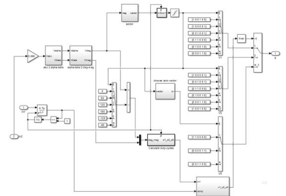
Fig -13: MC SVM symmetric switching for Rectifier Inversion matrix sequence of the SVM modulation when the voltage mod input to generate (v1-v2-v7- v8) with the switching pattern is constructed as in the Fig.14
