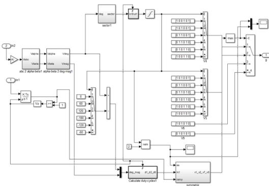
**Fig -14:** MC SVM symmetric switching for Inverter
