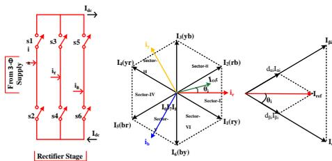
**Fig -6:** (a) VSR stage of of MC (b) Input current vector diagram in Hexagon form (c) Sector of VSR Hexagon
